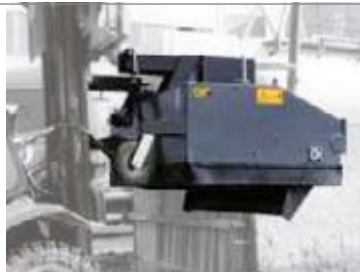
Collection bucket with tilt hydraulic cylinder
